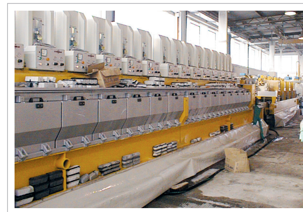
In line with cutting and chamfering machines In linea con attestatrici e bisellatrici
